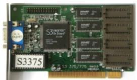
Core: 86C375 50,11 64bit Memory: 2/4MB EDO 50,11 64bit Year: 1996 Bus: PCI
