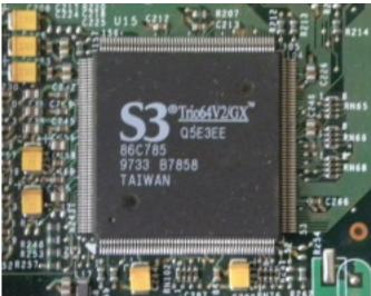
Core: 86C785 65MHz 64bit Memory: 2MB EDO 65MHz 64bit Year: 1996 Bus: integrated PCI
