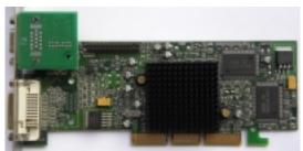
Core: MGA-G550-B 133MHz 128bit Memory: 32MB DDR 333MHz 64bit Year: 2001 Bus: AGP 4x Made: 180nm Pixel pipelines: 2 TMU per pipeline: 2 DirectX: 6.0 OpenGL: 1.1 Pixel write speed: 266 MPixel/s Texel write speed: 532 MTexel/s
