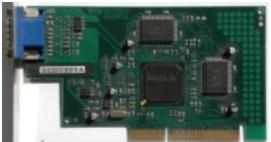
Core: MGA-G100A-E 40MHz 64bit Memory: 4MB SGRAM 60MHz 64bit Year: 1998 Bus: AGP 1x Made: 350nm
